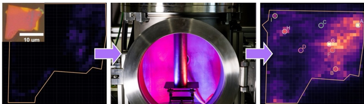
Fig. 1: (left) Optical microscope image of an hBN flake (inset) and its photoluminescence map, which shows only minute photoemission. Orange lines indicate the outline of the flake. After remote plasma exposure (center), individual emitters can be seen in the luminescence map (right).
